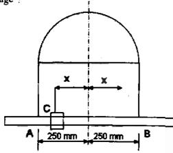
A homogeneous sphere weighing 10 kg is attached to a slender rod of mass 2 kg. If the system is released from horizontal position in rest condition, find the magnitude of angular acceleration. Also find angular velocity of system when it passes through vertical position,
